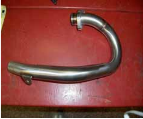
Left head pipe Figure 7
